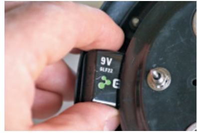
Pull battery out with fingers.
