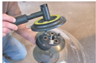
Center Handle onto stud.
