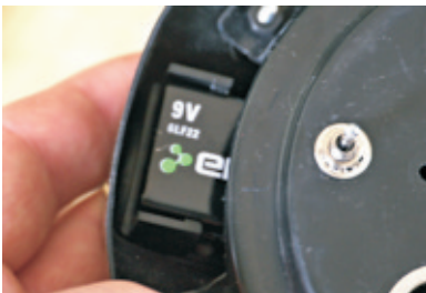
Seat battery into snap.
