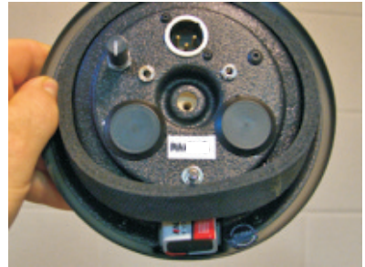
Move foam to access battery.
