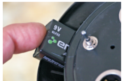
Push battery into place.
